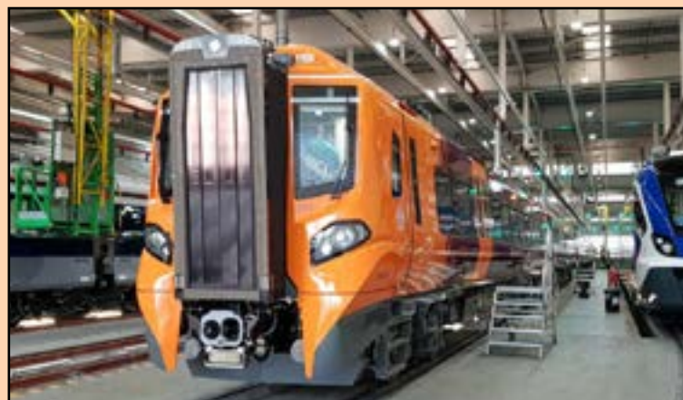
A Class 196 unit in production at CAF's factory in Newport.
